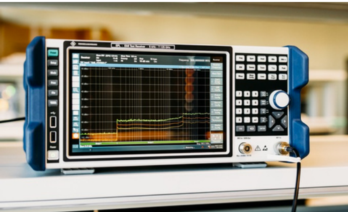
EMI Receiver used for measuring the electromagnetic emission spectrum.
