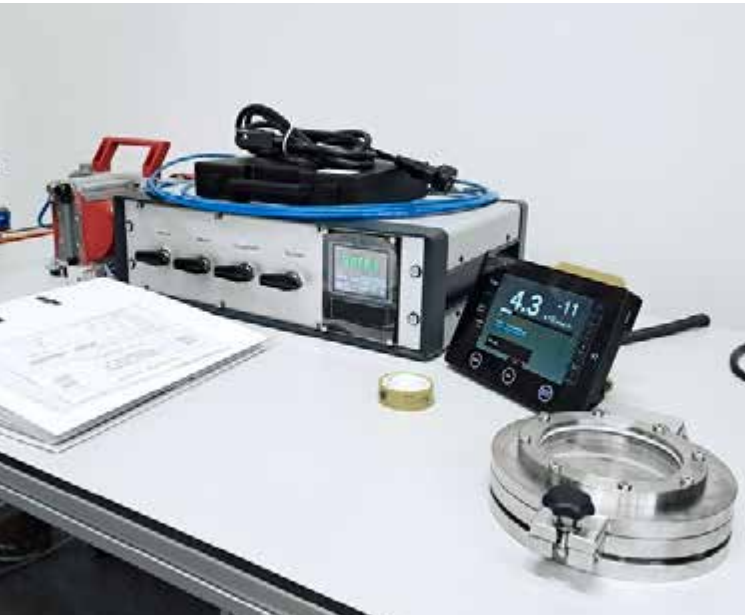
Custom-designed sealing tester with the pressure chamber (left side) and the chamber for leakage testing (on the right side).
