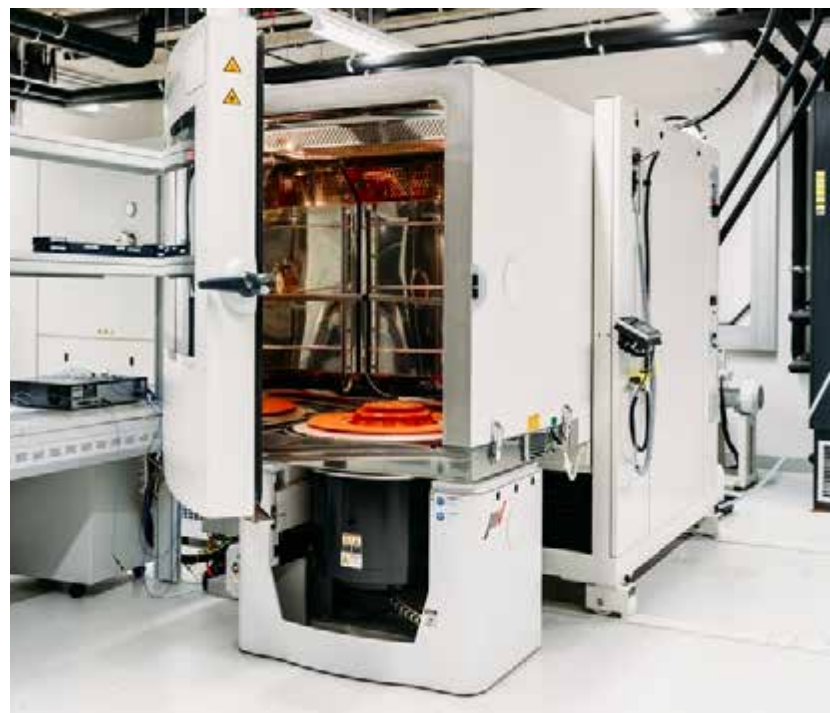
Climate Chamber combined with the Shaker
