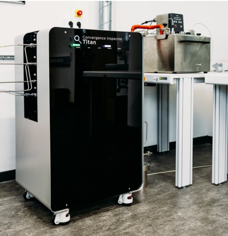
Gas Test Stand by DEMCON Convergence with machine part (left) and sample chamber in water bath (right)
