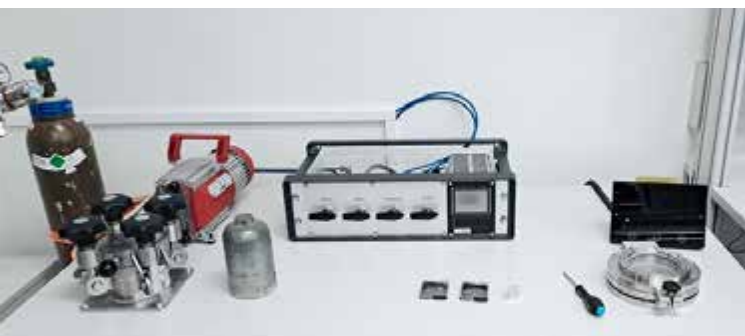
Custom-designed sealing tester with the pressure chamber (left side) and the chamber for leakage testing (on the right side).
